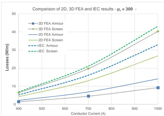
Fig. 10: Comparison of screen and armour losses. Magnetic permeability  $\mu_r = 300$
