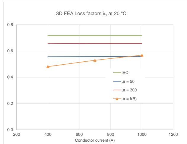
Fig. 11: Loss factor  $\lambda_1$  calculated with 3D FEA
