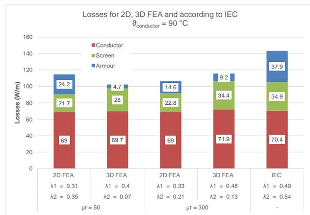
**Fig. 8: Comparison of simulated and estimated losses for temperatures of 90 °C, (conductor) 80 °C (screen) and 60 °C (armour)**
