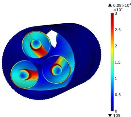
**Fig. 6: Calculated distribution of three-dimensional loss density (W/m<sup>3</sup>) μ<sub>r</sub> = 50**
