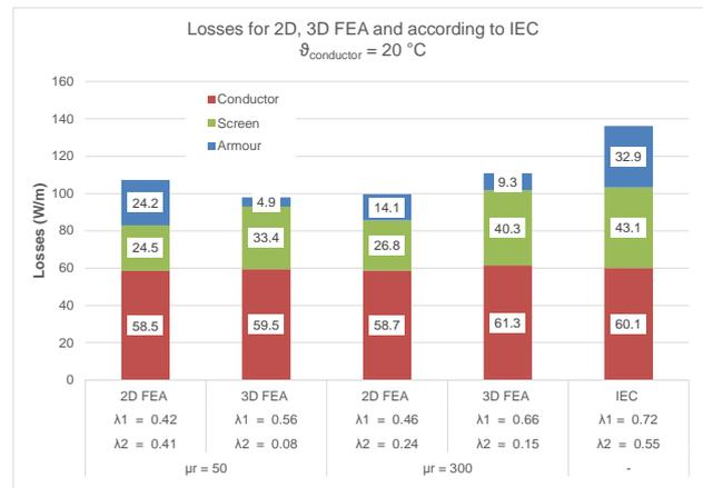
**Fig. 7: Comparison of simulated and estimated losses for an overall temperature of 20 °C**
