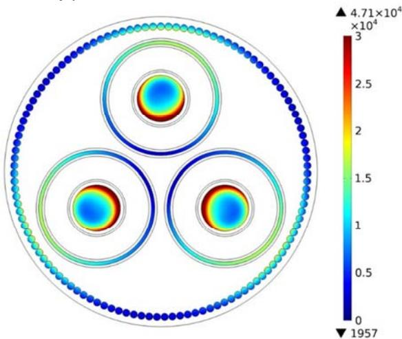
**Fig. 5: Calculated distribution of two-dimensional loss density (W/m<sup>3</sup>) T = 20 °C; μ<sub>r</sub> = 50**
