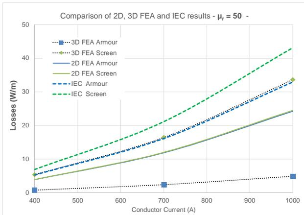
Fig. 9: Comparison of screen and armour losses. Magnetic permeability  $\mu_r = 50$
