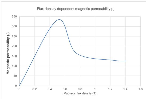
Fig. 2: Permeability as a function of magnetic flux density
