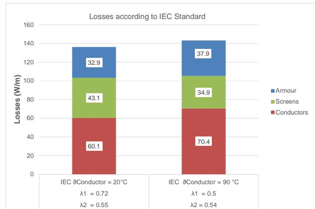
Fig. 4: Losses in a three-core submarine power cable<sup>1</sup>
