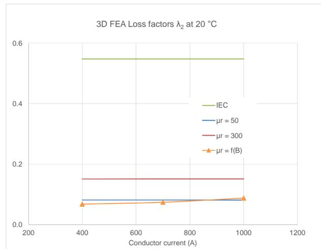
Fig. 12: Loss factor  $\lambda_2$  calculated with 3D FEA
