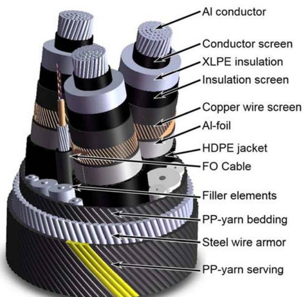
**Fig. 1: Schematic drawing of the submarine power cable design.**
