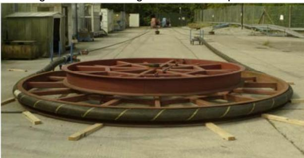
**Fig. 7: Tensile bending test of the 3x 800 mm<sup>2</sup> 19/33 (36) kV XLPE submarine power cable around a 5.4 m sheave.**
