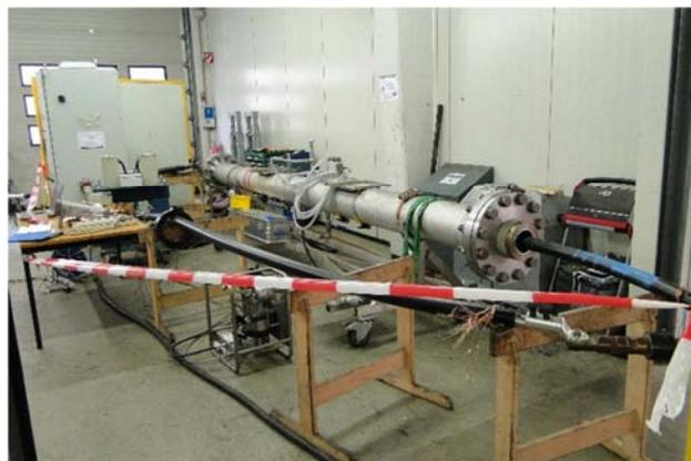
Fig. 9: Longitudinal water penetration test setup on the metallic screen of the power core.
