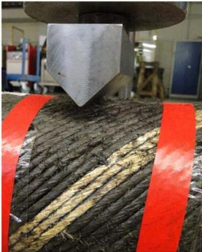
**Fig. 3: Impact Test, the impact hammer had a curvature radius of 2 mm.**
