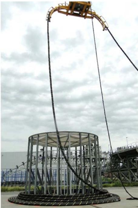
**Fig. 6: Coiling test of the 3x 800 mm<sup>2</sup> 19/33 (36) kV XLPE submarine power cable into a fixed static tank**
