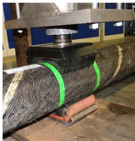
**Fig. 2: Crush test with original caterpillar track pads**
