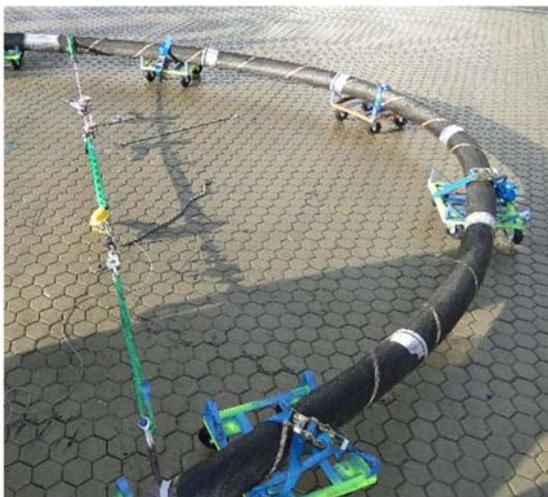
**Fig. 4: Test arrangement to measure the bending moment and curvature to investigate the bend stiffness.**
