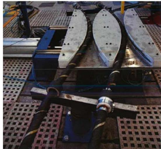
**Figure 2: Bending against template test arrangement
